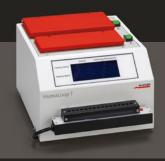
**HumaLoop T** (incubator for sample processing, amplification and visual result reading) **REF:** 961000
